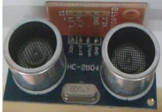
Figure.7.Schematic Diagram for Ultrasonic sonar sensor
