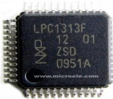
Figure.5. ARM7 LPC1313 Microcontroller B) L293D DRIVER
